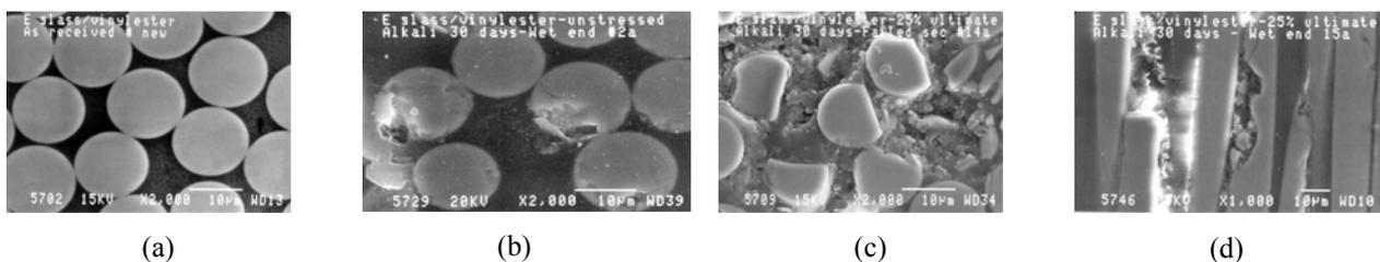
Figure 1. Scanning electron micrographs of GFRP with vinylester resin with the condition of (a) as received and exposed to alkaline environment as well as (b) unstressed after 30 days, (c) stressed to 25 % of ultimate tensile strength after 30 days and (d) its longitudinal failed section (Rajan et al., 2002)
