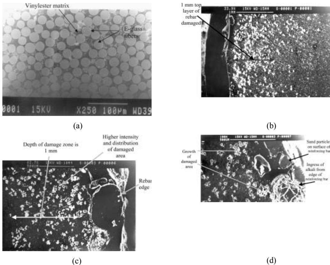
Figure 2. Scanning electron micrographs of (a) original GFRP bars and of damage near bar surface conditioned in 60°C alkali solution for (b) 3 months, (c) 6 months and (d) 12 months (Mukherjee and Arwika, 2005)
