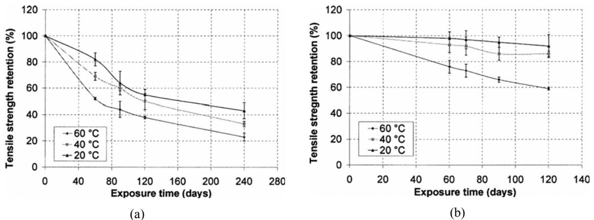
Figure 3. Tensile strength retentions of (a) GFRP1 and (b) GFRP2 bars exposed respectively to solution 1 and 2 at 20, 40 and 60 °C (Chen et al., 2006)
