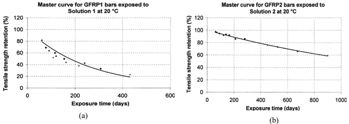
Figure 5. Tensile strength retention versus exposure time for (a) GFRP1 and (b) GFRP2 bars (Chen et al., 2006)
