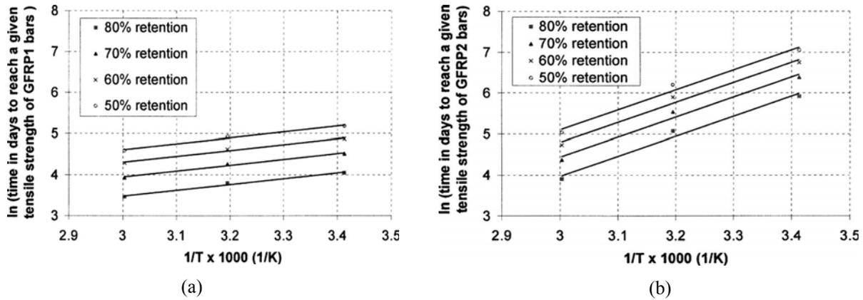
Figure 4. Arrhenius plots of tensile strength degradation for (a) GFRP1 and (b) GFRP2 (Chen et al., 2006)
