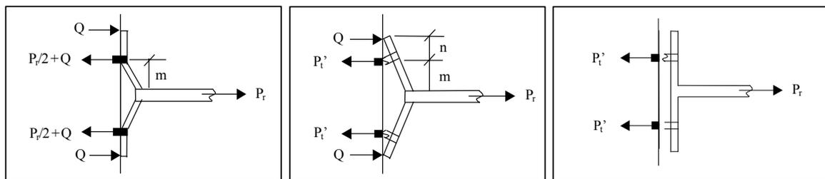
(a): Type 1 Complete flange failure. (b) Type 2 Bolt failures with flange yield (c) Type 3 Bolt failure.
