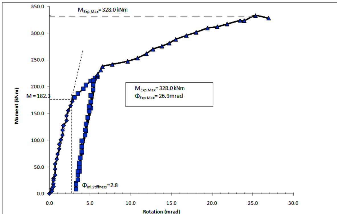
Figure 8 Moment vs rotation for EEP 3.
