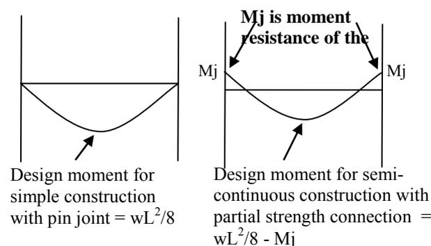
Figure 1: Design moment for beams due to different support conditions
