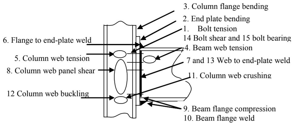
Figure 4. Critical zones that need to be checked for failure
