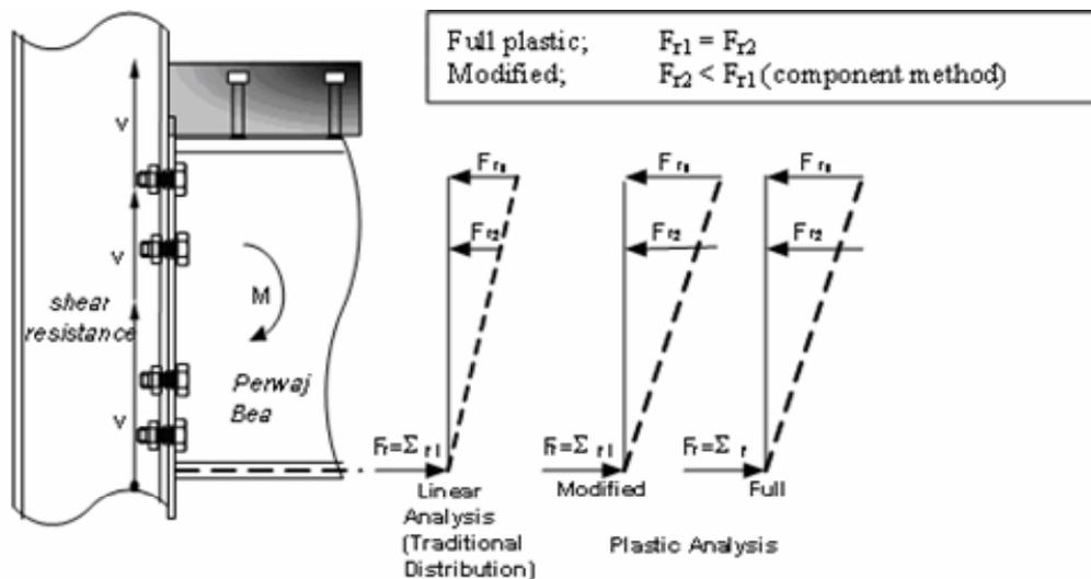
Figure. 5 Elastic and Plastic Analysis of Bolt Forces Distribution in Composite Connection
