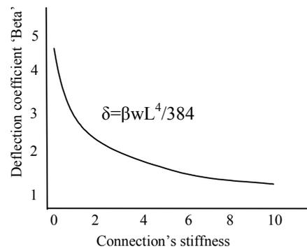
Figure: 2 Deflection coefficient 'Beta' as a function of relative stiffness of connection
