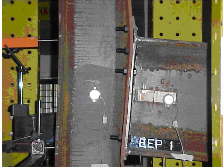
Figure 9. Deformation of end-plate and column flange in tension zone.
