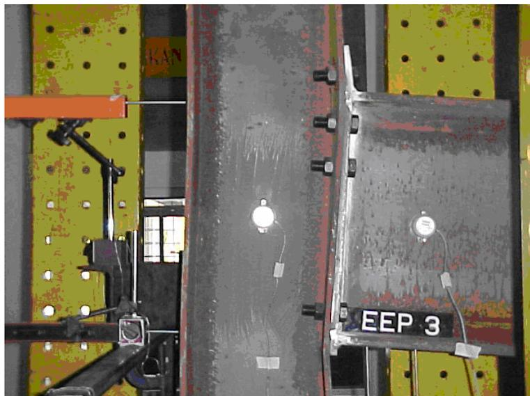
Figure 10. Deformation of end-plate and column flange in tension zone.
