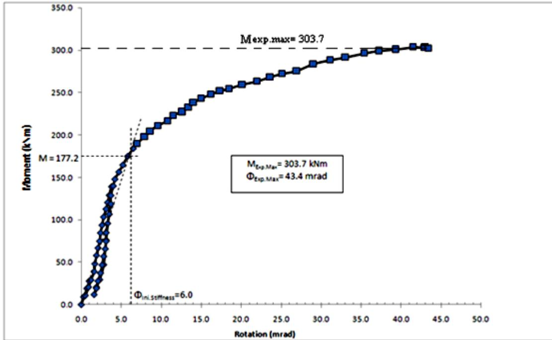
Figure 7 Moment vs rotation for EEP 1.
