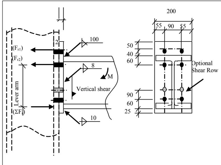
Figure 3: Typical extended end-plate connection.
